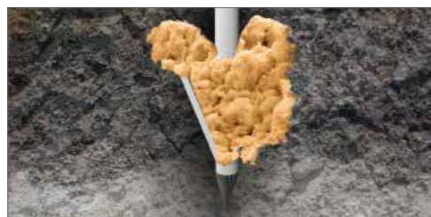
B07. Foam harpoon ejecting foam into the asteroid's soil.
