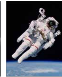
B02. Astronaut performing an EVA using the Manned Manoeuvring Unit.
