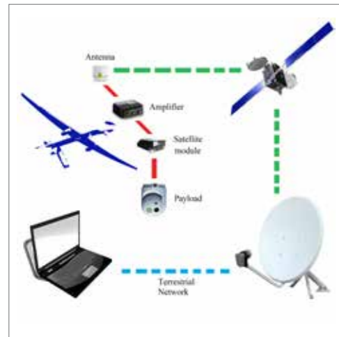
3. UAS schema for the communication system
