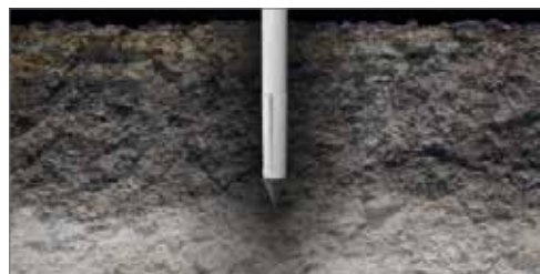
B06. Foam harpoon penetrating the asteroid's soil.
