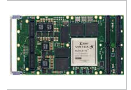
9. FPGA Virtex5 by Xilinx®
