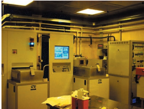
10 31/10/2006, Lecce. Visit to the National Nanotechnology Laboratory. Clean Room: in this protected environment the number of particles in each \text{cm}^3 of air is kept below a fixed threshold. It is used for lithographic processes.
