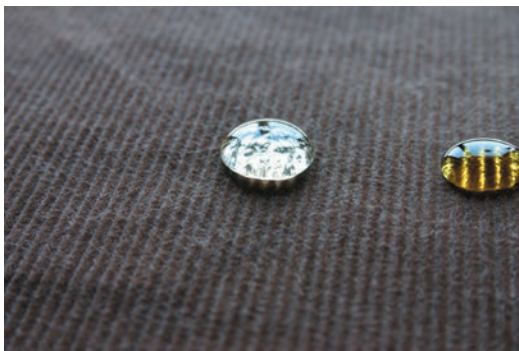
7 Drops of honey and olive oil on the nano-treated fabric: both maintain a round, closed form
