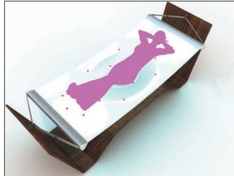
8 Distribution of the sensors inside the cloth
