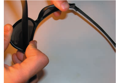
6 Prototype consisting of a pair of NXT soft 54 lenses and a silicone rubber frame
