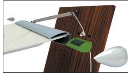
12 Exploded view of the hanging system: the plastic cap, the elaboration unit, wires, the extruded aluminium component, the cloth
