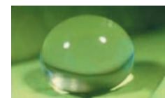
4 The droplet only touches the super-hydrophobic surface at a few points and due to its surface tension, forms a sphere
