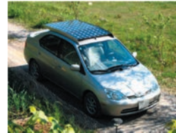
11 The roof of this car is equipped with solar cells
