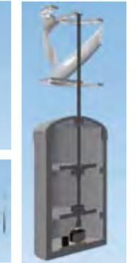
14 3D rendering of the turbine system (exploded view)
