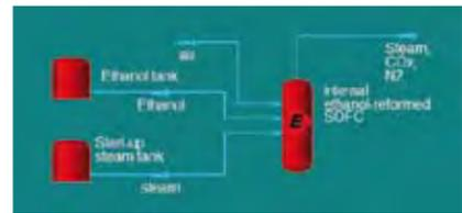
6 Pure Wings proposal: an internal ethanol-reformed SOFC coupled with an on-board ethanol tank and a start-up steam tank
