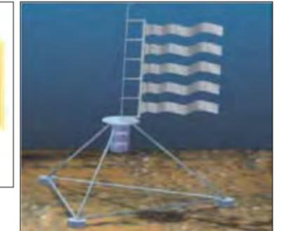
4 Idea for a tidal flow converter based on an array of piezoelectric eels. Author: Ocean Power Technologies - Pennington, NJ
