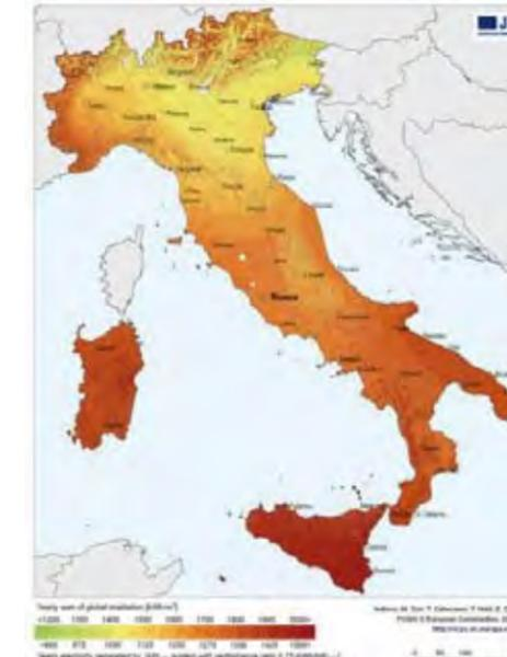
6 Global irradiation and solar electricity potential for optimally-inclined photovoltaic module in Italy
