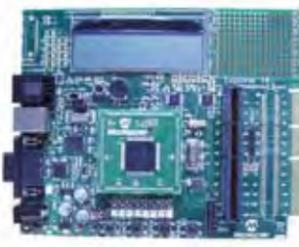
4 Evaluation board with the microcontroller used in the control unit
