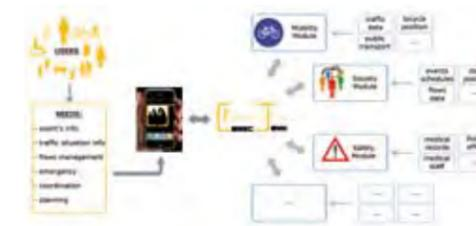
6 Platform structure. Three modules collect data from different institutions and sources (existing databases, real-time anonymous data and user-generated content). These resources are processed by the platform. Users can seamlessly access these resources through a mobile phone application or other devices. The modular structure allows an incremental implementation strategy.
