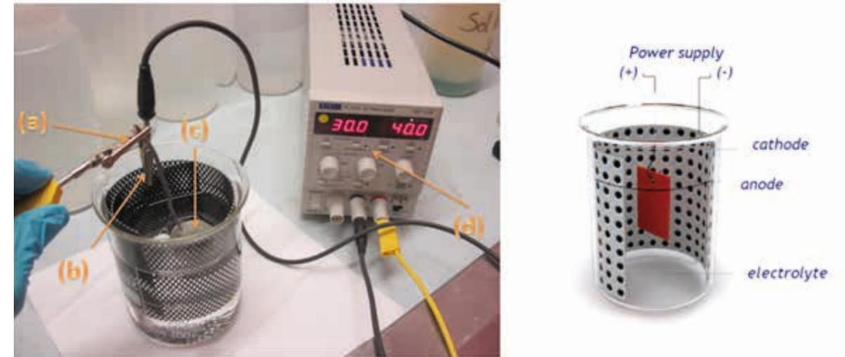
Setup of the anodization
