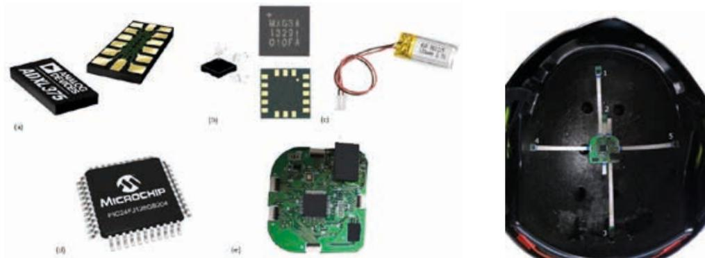
Electronic components of the integrated circuit. (a) linear accelerometer (b) gyroscope (c) LiPo battery (d) microcontroller (e) FLASH memory.
