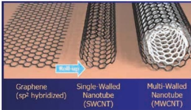
Model of a single-walled carbon nanotube (SWCNT) as obtained from a graphene sheet. Multi-walled carbon nanotubes (MWCNTs) are obtained through rolling of some overlapping sheets
