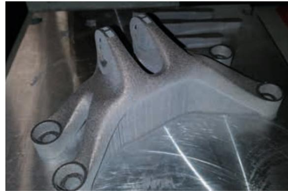
Printed bracket with support structure
