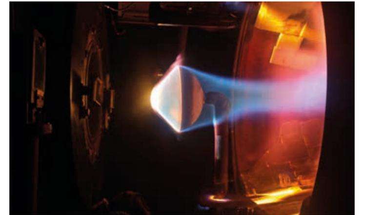
Experimental test in hypersonic plasma jet to verify materials behavior under reentry conditions.
