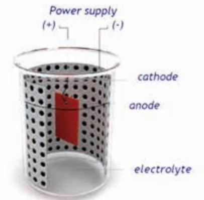
Setup of the anodization
