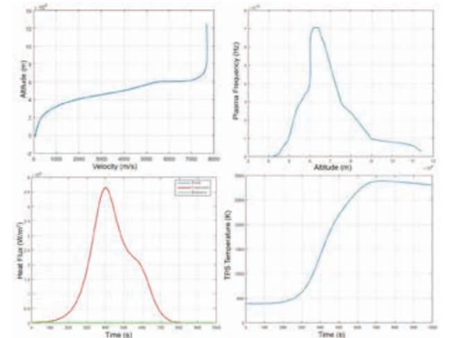
Plots of some of the outputs from the code. The Velocity, the Plasma Frequency, the Heat Flux and the TPS temperature are represented during the reentry phase conditions.
