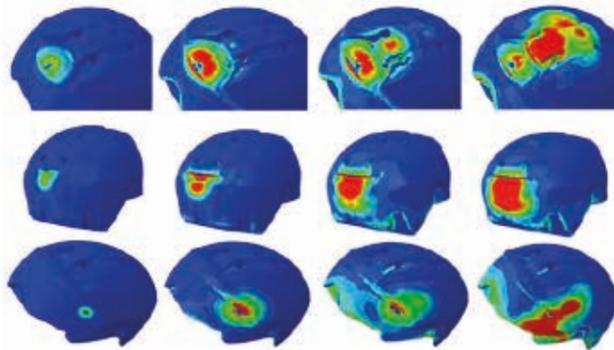
FEM results of stress field of external surface of EPS foam at 0, 0.5, 1, 1.5 and 2 ms. Top: upper impact, middle: rear impact, down: lateral impact. Max stress=0.5 MPa (traction, in red), Min stress=1 MPa (compression, blue)
