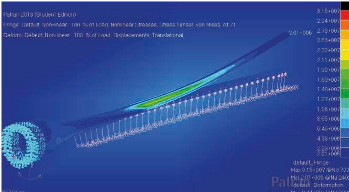
Non-linear static analysis showing stresses with the VM criteria for the not-optimized thickness GFRP configuration
