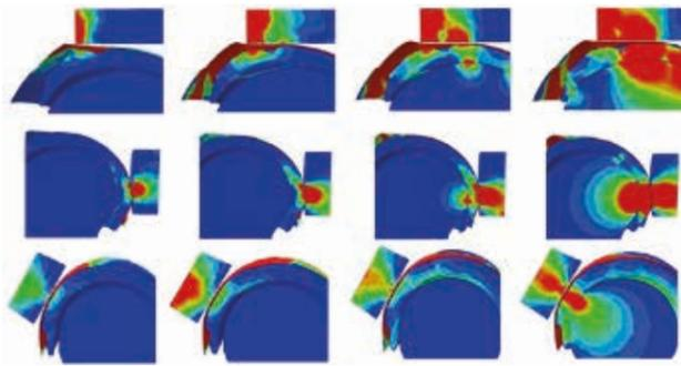
FEM results of wave propagation across the layered thickness at 0, 0.5, 1, 1.5 and 2 ms. Top: upper impact, middle: rear impact, down: lateral impact. Max stress=0.5 MPa (traction, in red), Min stress=1 MPa (compression, blue)
