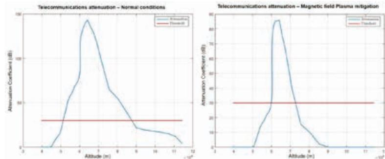
Plots showing the effect of the magnetic field on telecommunications. When it's not applied, the radio-frequency blackout is experienced between 90 and 50 km of altitudes. If the mitigation approach with magnetic field is applied, the duration of the blackout is shortened between 75 and 60 km above the Earth.
