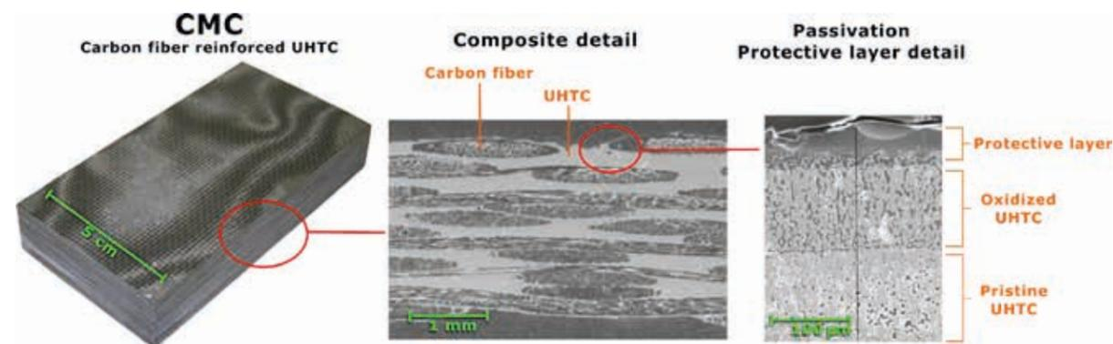
Proposed material design for the heat shields. Picture of different scale, showing composite structure and protective layer produced by the material when exposed to high temperatures.
