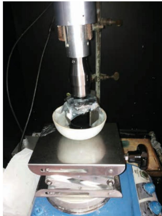
Image of the ultrasound technique arrangement during mixing.
