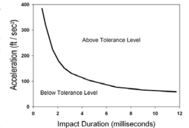
Hyperbole identifying impact over tolerance level according to acceleration and duration, by Greenwald et Al. [2].
