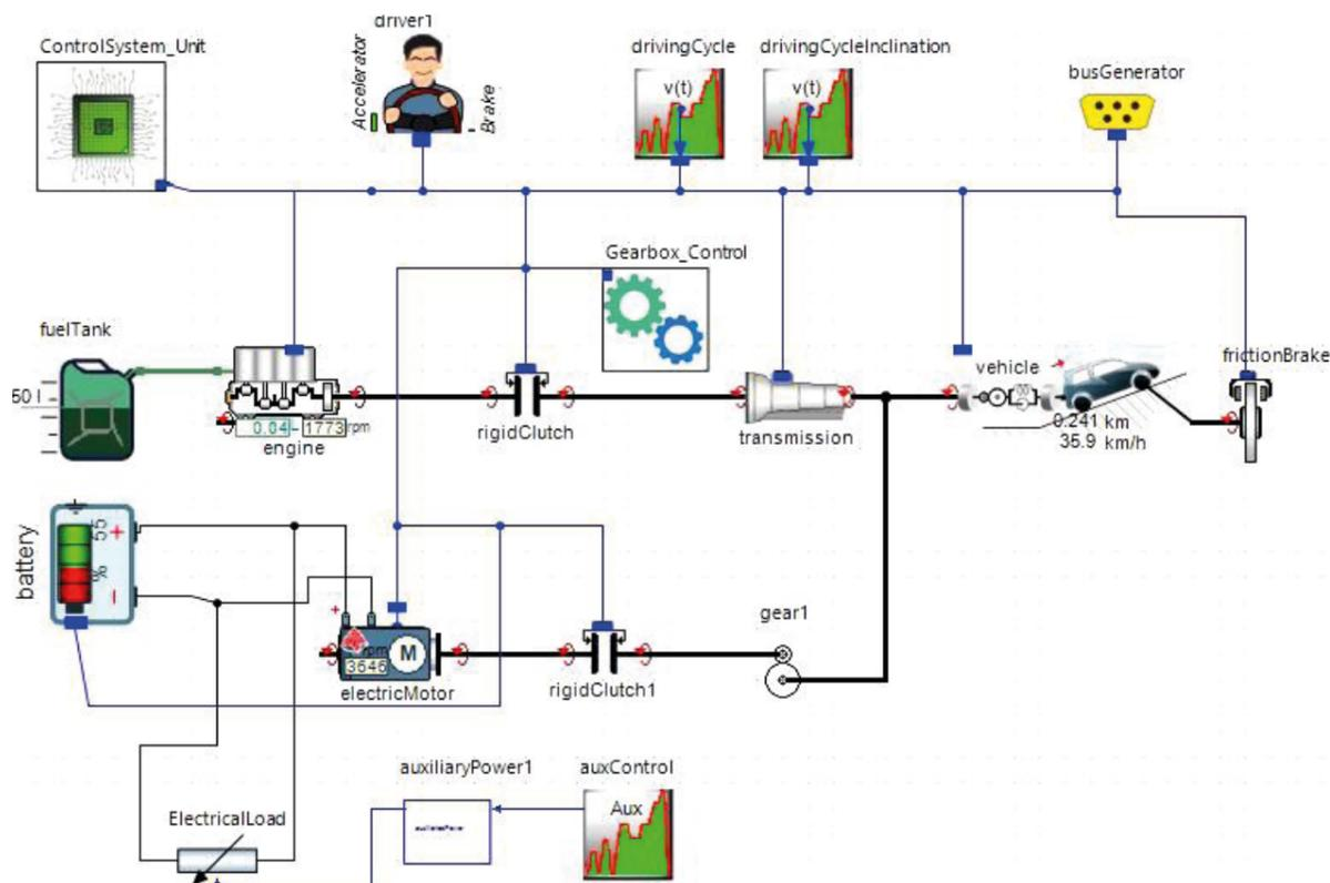
Once an effective virtual tool has been created, several control logics and configurations have been tested, aiming on the reduction of pollutants and the increase of the vehicle efficiency.
