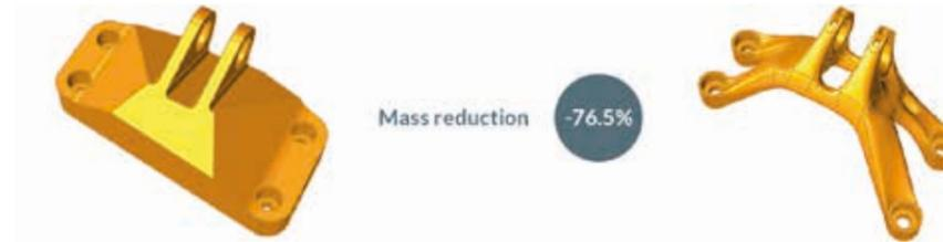
The original part object of the case study (on the left) and its optimized version (on the right)
