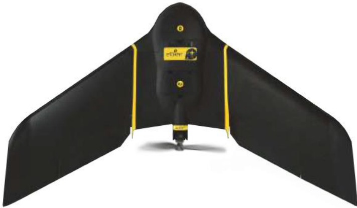
Figure 7 - SenseFly eBee Plus for direct photogrammetry
