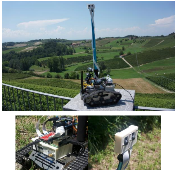
Figure: The prototype (above) and details: GPS box (down left) and the camera box (down right)
