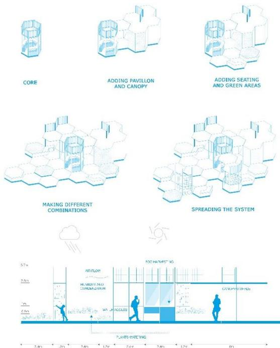
Various configurations may be arranged. An element always present in each configuration is the core, that represents the main fog collector. With every single hexagon module, we wanted to include different functions, so they correspond to individual users.
