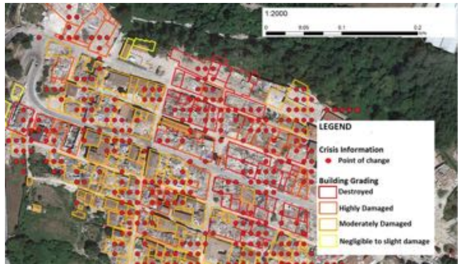
The result of a run of the algorithm (red points) over the Amatrice earthquake in comparison with the European Space Agency building damage grading (structure shaped geometries with four different building grading)
