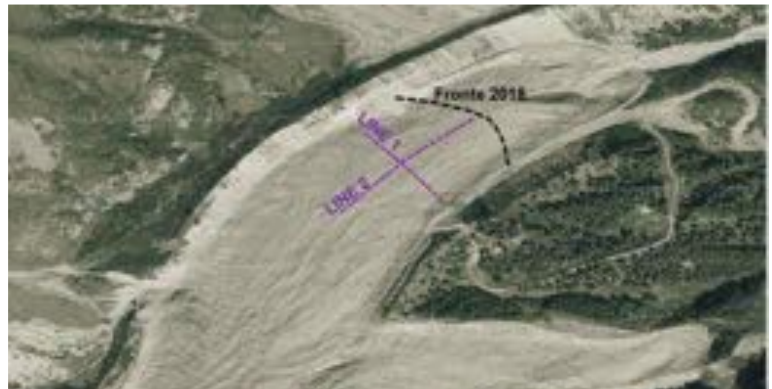
Figure 11 - glacier's sections investigated with geophysical surveys
