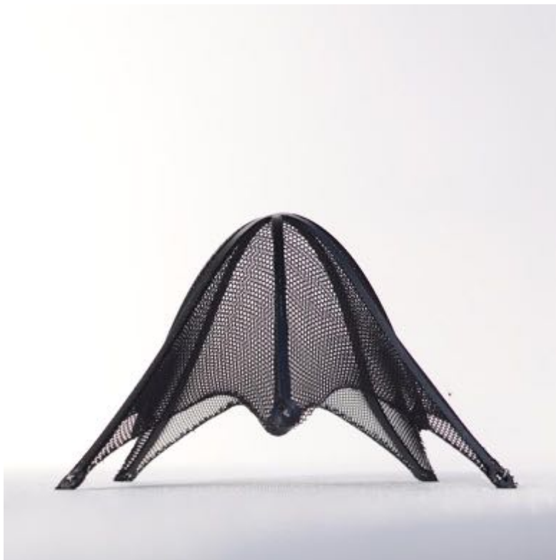
Photo of dome prototype exhibiting positive Gaussian curvature
