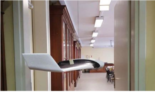
Figure 9 - Final solution: balancing test
