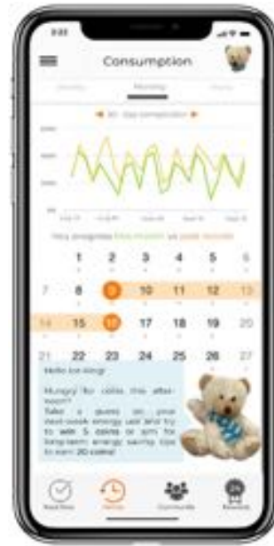
Figure 4: A comparison between current energy use and previous trends in the household is displayed in a graph. The users can choose which time frame to use for the comparison. Dr. Bear's pop-up messages keep the customer engaged.
