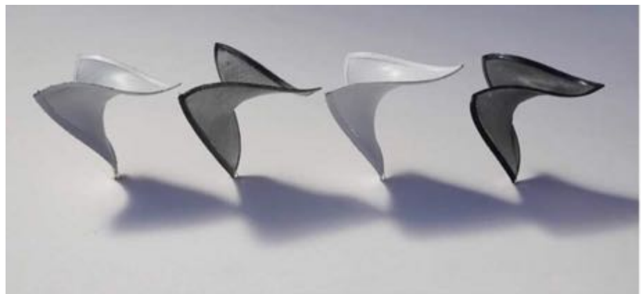
Four 'Hypar' prototypes after being coated; each exhibits slightly different structural characteristics based on the coating material
