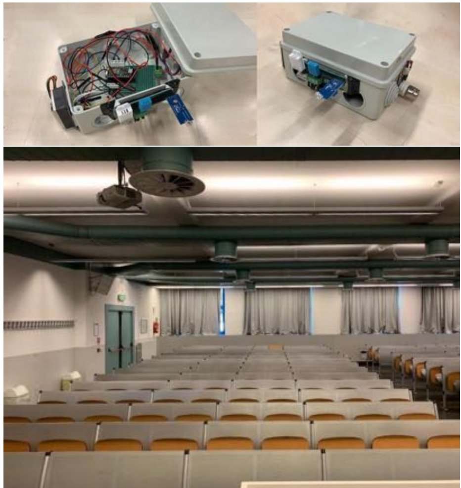
Figure 3. The first prototype of the thermostat installed in Emilio Gatti Conference room.
