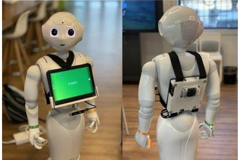
Figure 3: Our prototype, Pepper with the additional equipment (camera + backpack)
