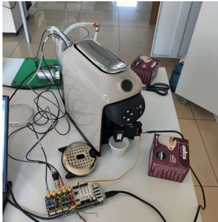
Physical prototype: IoT system embedded in Nespresso's coffee machine
