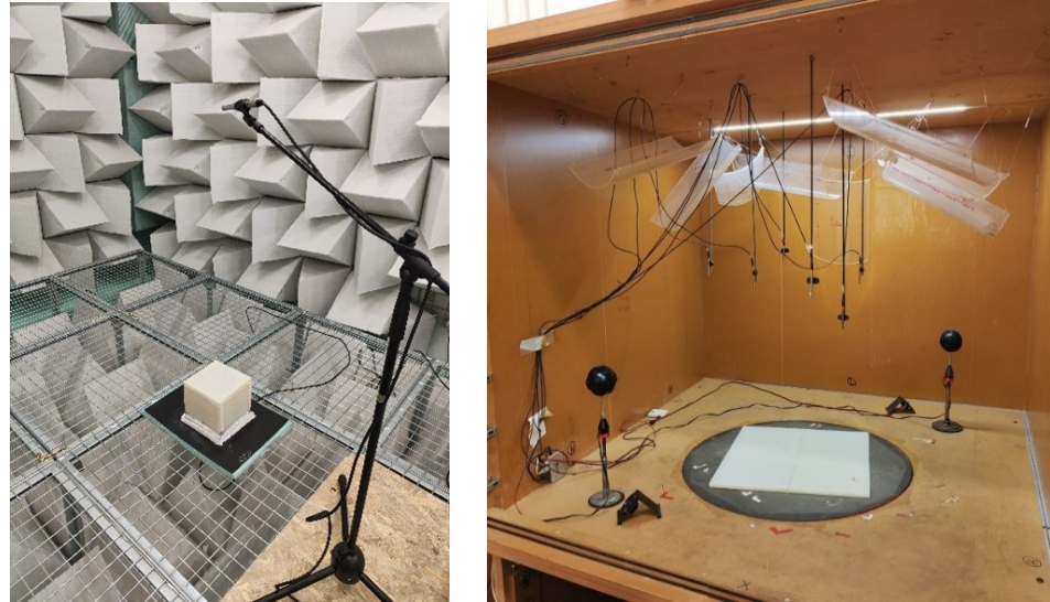
Figure 6: Experimental setups for the cubes (insertion loss) and the panel (absorption) acoustic performance measurements.
