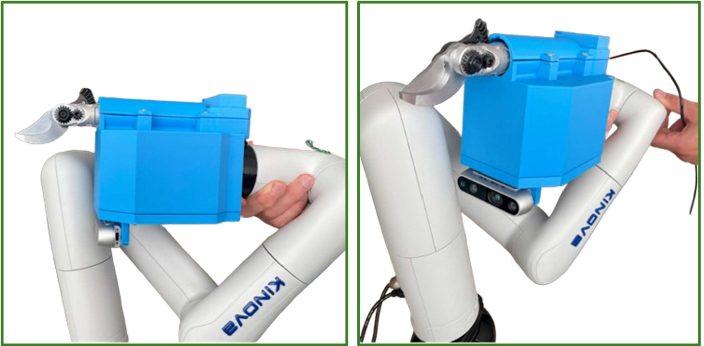
Figure 1: Robotic pruning end-effector mounted on Kinova Gen3 Lite arm.
