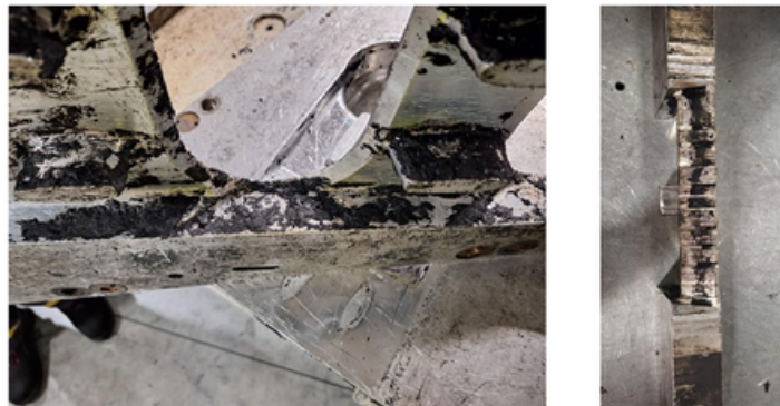
Image of the head cleaning problem after a production cycle
