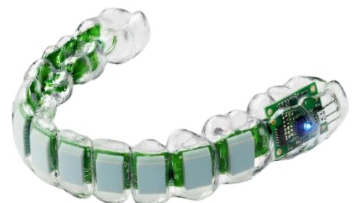
Fig. 3 Sensorized Dental Aligner: the integrated PCB is shown in green and the pressure sensors in light blue. The electronic components are ultra-thin and flexible, conforming seamlessly to the aligner's shape without compromising fit or comfort.
